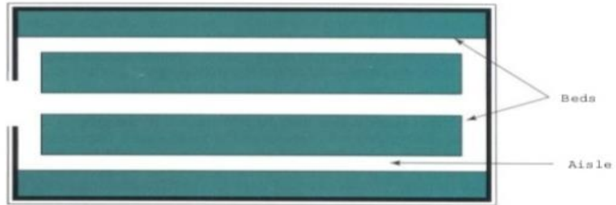
Longitudinal layout of polyhouse beds
